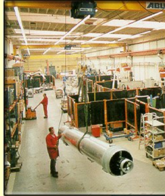
Production shop for busducts, showing machines, welding bays
