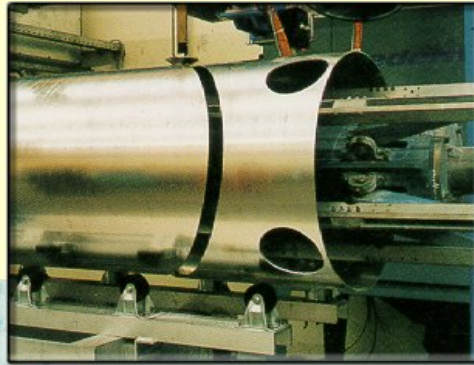
CNC plasma cutting machine for round cuts and cut-outs in the enclosure
